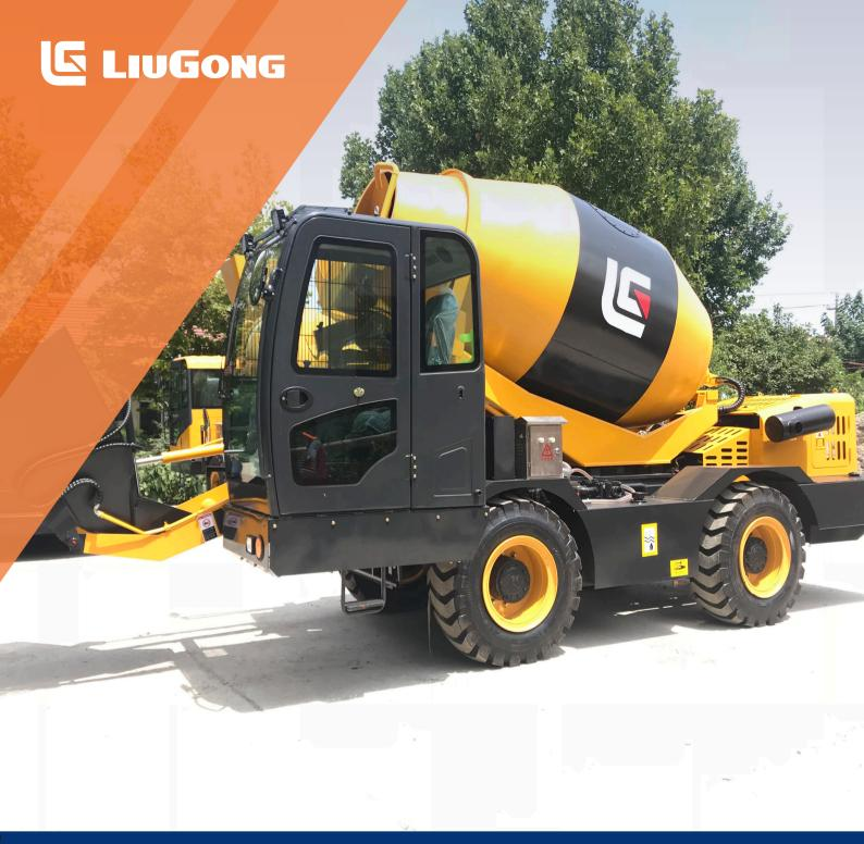
Engine Brand Emission Regulation Drum Capacity Transmission Chassis Driving Type Rotation Angle DCEC Optional 4 m<sup>3</sup> Full Hydraulic 4WD,2WS 270°
